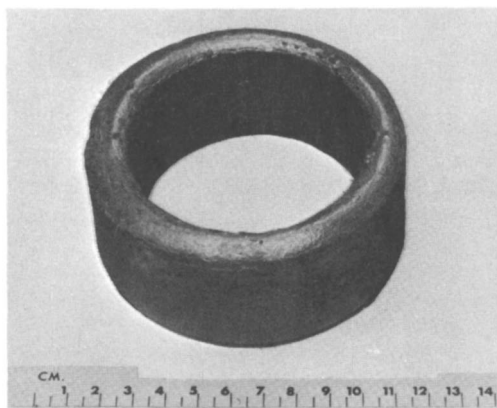
Figure 9. Typical electrorefining product ring.
