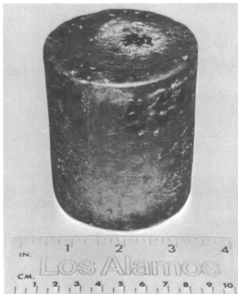
Figure 6. Impure metal ingot feed for electrorefining.
