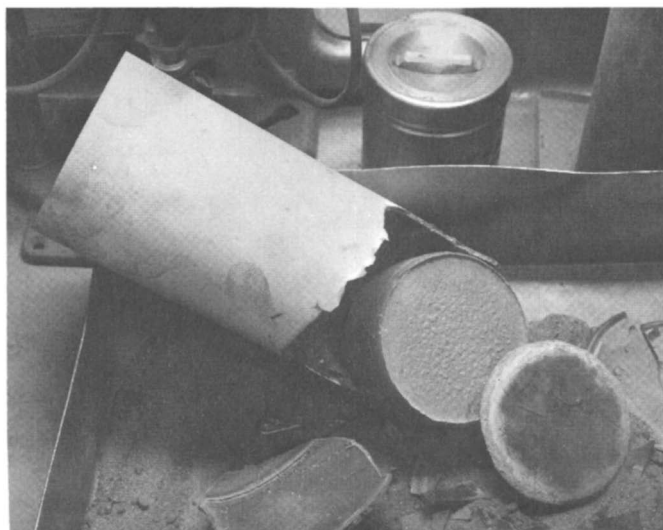
Figure 5. Plutonium tetrafluoride reduction slag and product metal.
